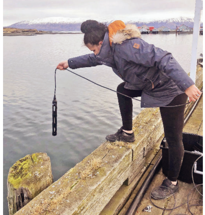
Jamie Hubbard using a water sampling instrument to gather temperature, salinity, dissolved oxygen, and pH levels in Larsen Bay.
